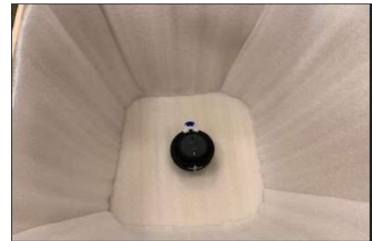
Bluetooth Speaker Placement in Material Lined Wood Box
