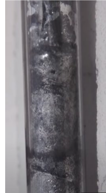
Deposit of solid carbon on the side of the CO 2 bubbling tube and on the surface of bubble column
