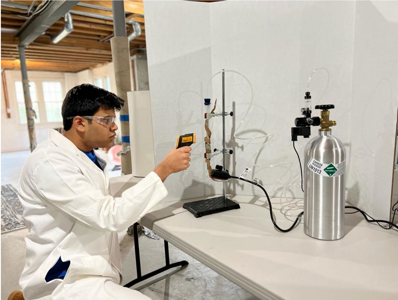
CO 2 flow rate controlled via needle valve and bubble rate measurement Temperature controlled via infrared measurement and a heating tape
