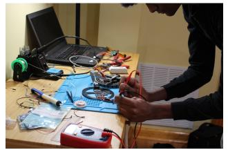
Testing the boost converter for the first time to see if it would output a 60v current
