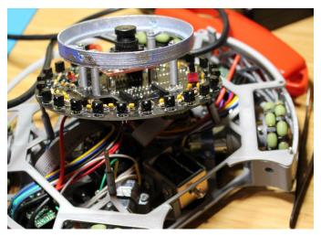
While designing the PCB I prioritized through-hole components as it would be easier to hand solder.
