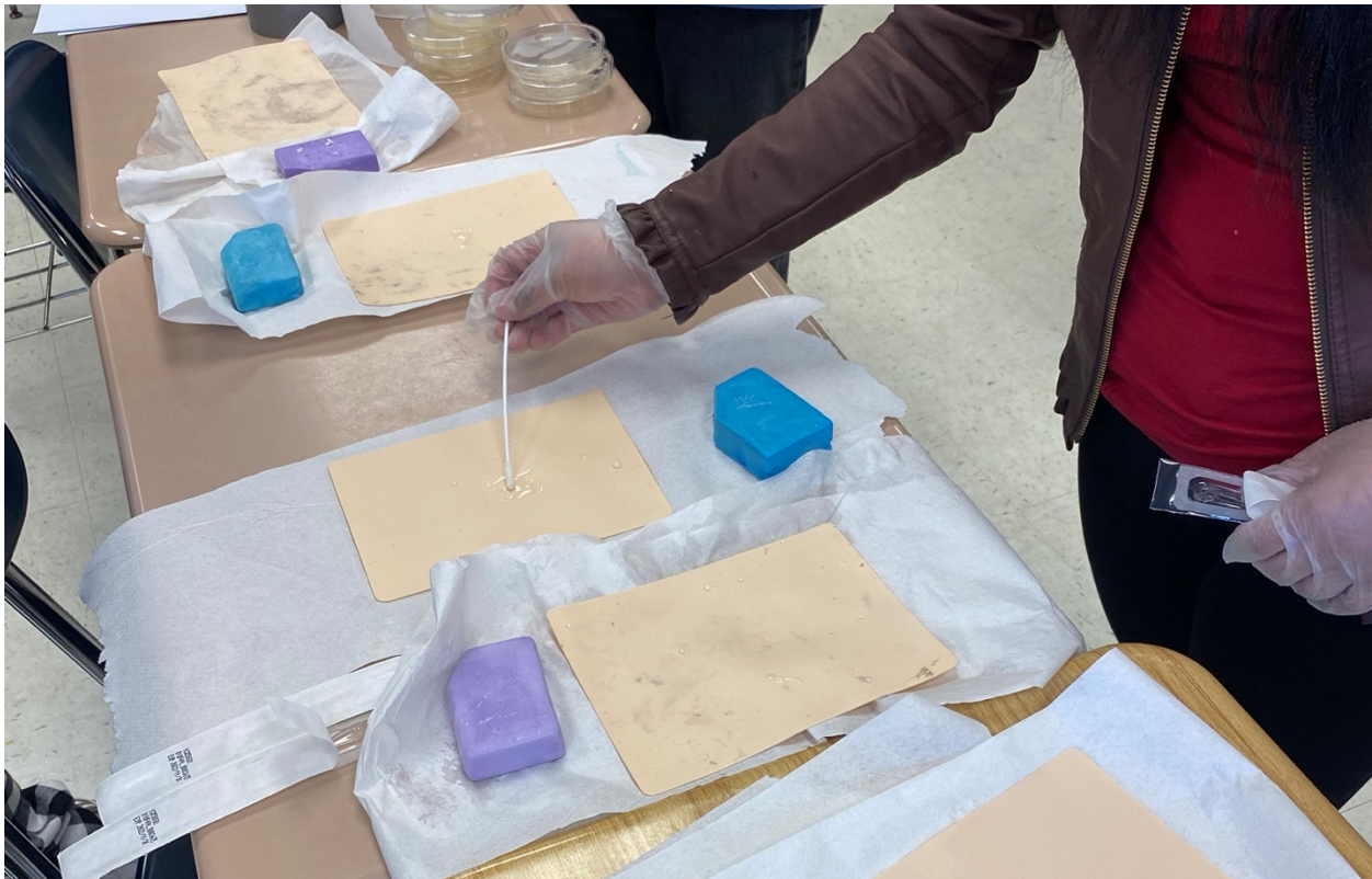
Figure 6. Disinfecting trials with 0.1 mL of E. coli var. K-12 being spread on a 1.0 x 1.0 cm patch of artificial silicone skin. After the bacteria was placed on each sample, it was washed for 30 seconds with water and lather from the soap of choice, except for the controls. These skins were then swabbed and any
