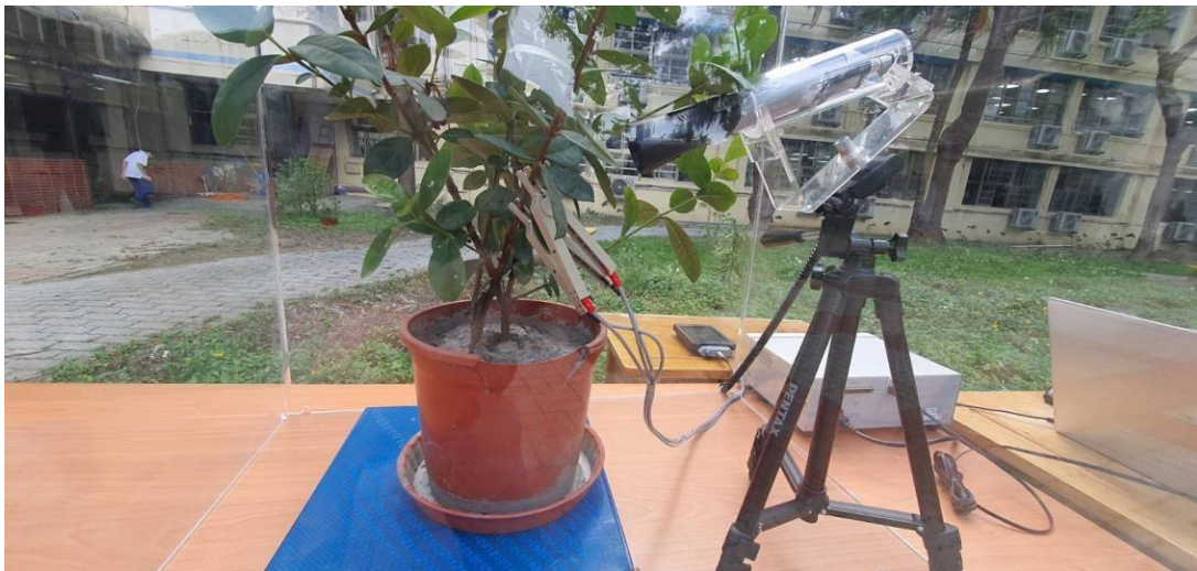
Fig. 9 Experiment setup surrounded by acrylic cover to minimize interference
